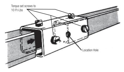
4.2.1 Track joints clamp for secure attachment and proper alignment of track section. Each kit includes four set screws and nuts.
