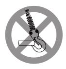
Can't hang the weight directly on the hook tip
