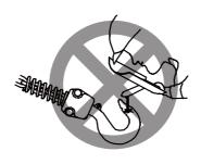
forbidden to weld the hook and the lifting chain
