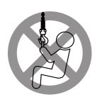
Hoist can not transfer Human being or use as Supporting mechanism
