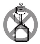
do not use lifting chain as have duty rigging
