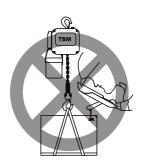
Forbidden to do welding or cutting operation when the weight was lifted in the air. **<u>∧</u>WARNING**
