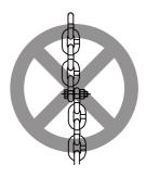
do not use bolt, screw screw driver etc to knot or shorten the lifting chain
