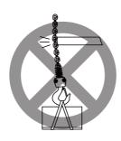
do not let the lifting chain pass through the obstacle surface such as steel plate
