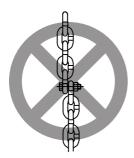
do not use bolt, screw screw driver etc to knot or shorten the lifting chain
