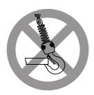
Can't hang the weight directly on the hook tip
