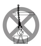
do not let the lifting chain pass through the obstacle surface such as steel plate
