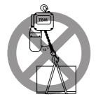
do not lift the goods slant the angle can not over 12 than vertical direction
