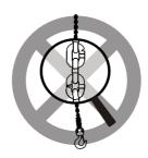
Forbidden to use the hoist which has deformation or crack in lifting chain
