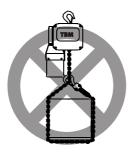
do not use lifting chain as have duty rigging
