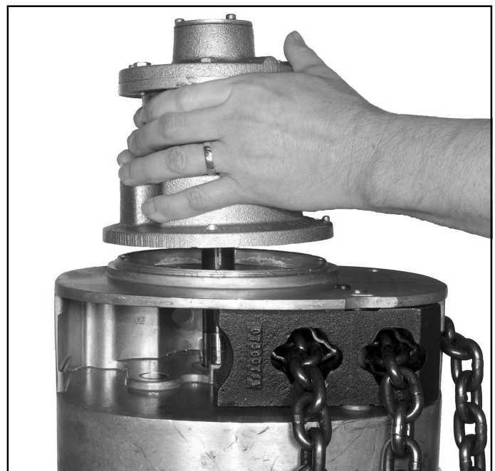
Figure 7-8. Removing Motor Assembly
