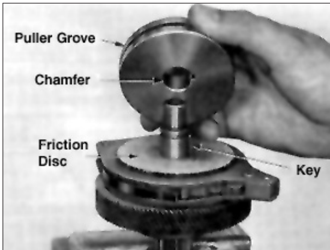
Figure 5-7. View Showing Load Brake Flange Removed
