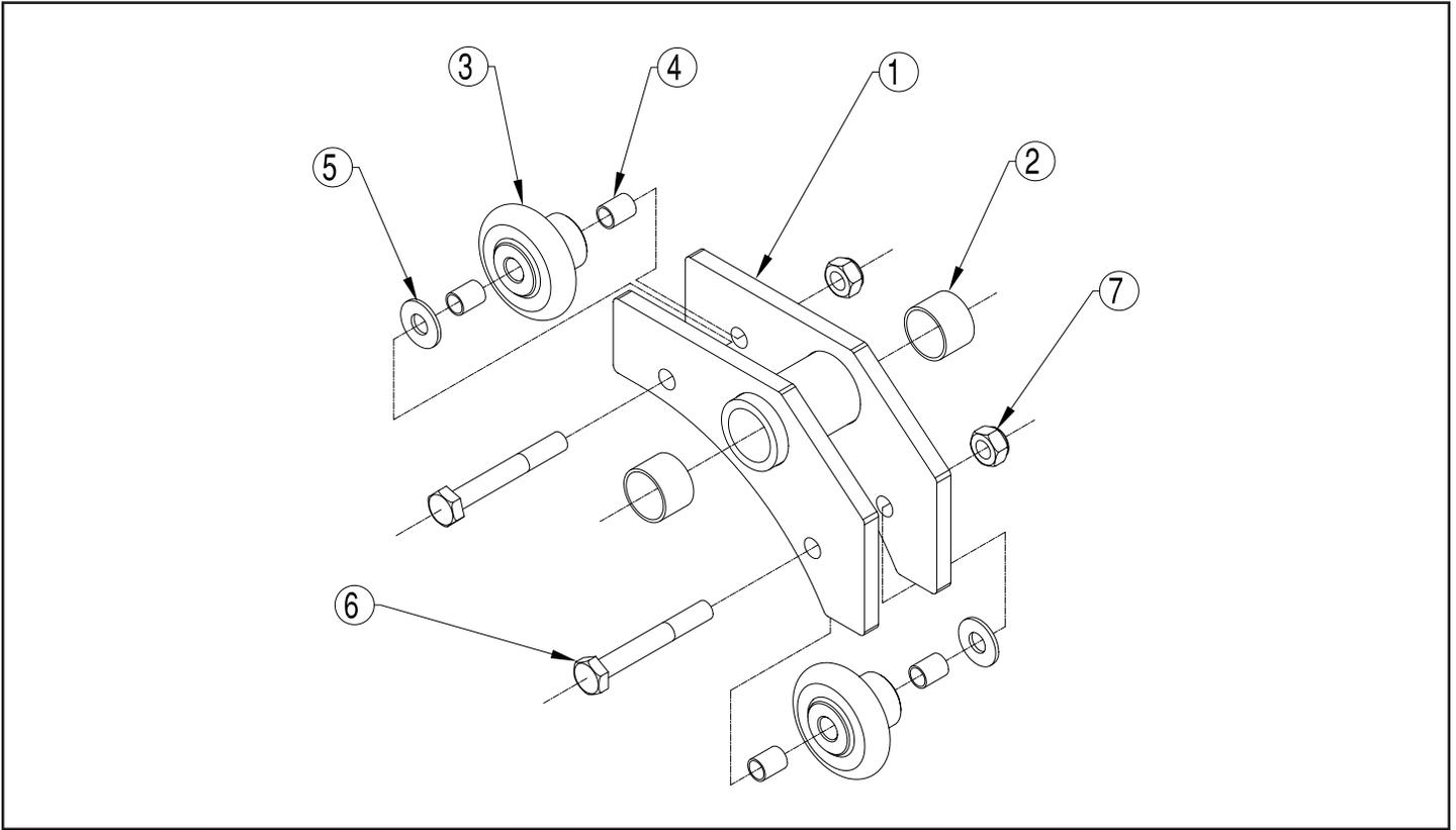
Figure 9-7b. Rope Guide Assembly (S4 & S2 Reeved)
