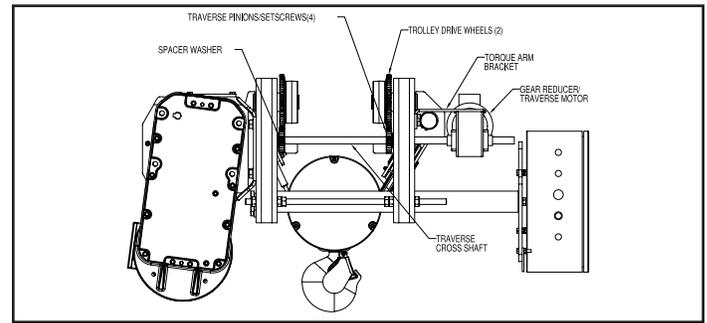
**Figure 5-9. Traverse Drive Arrangement ("B" & "C" Frame Shown)**
