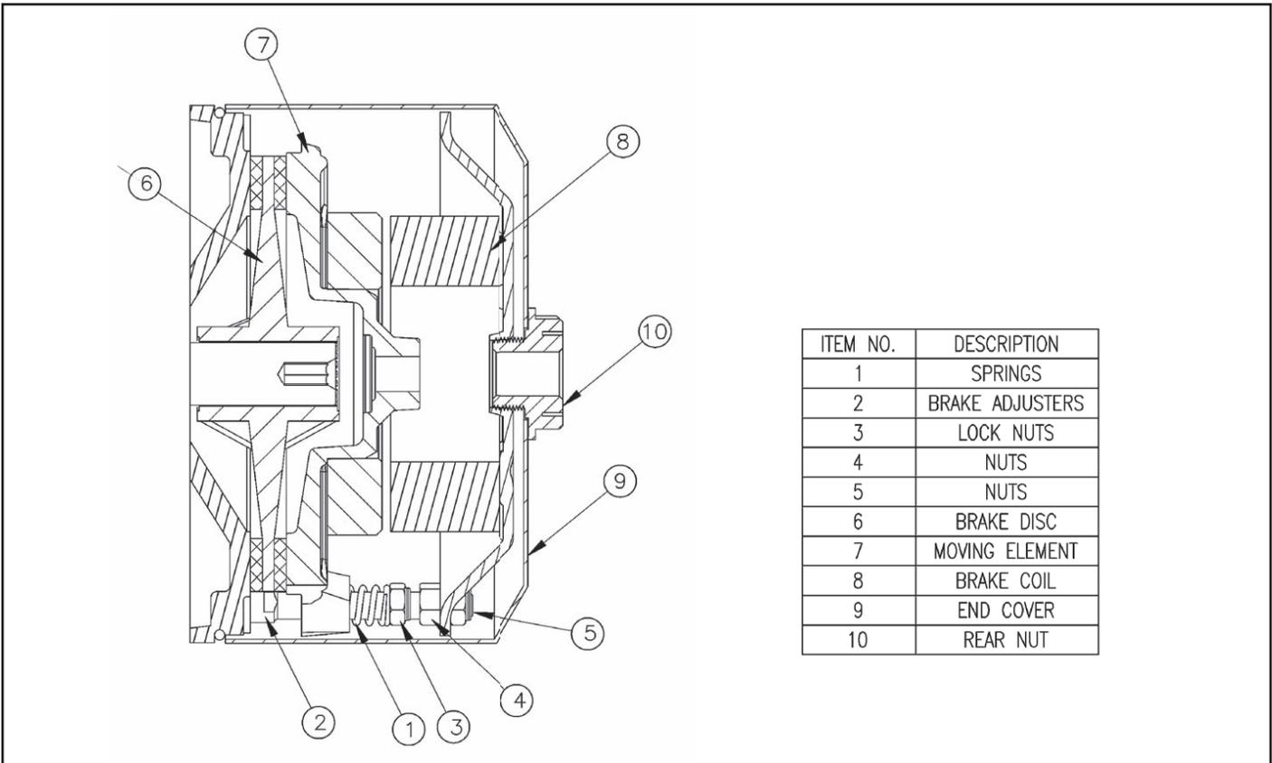
Figure 9-10a & 9-10b. Standard Hoist Motor Brake (MGM Motor)
