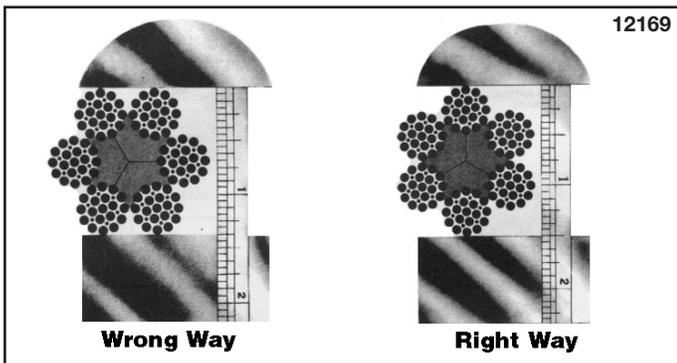
**Figure 5-4. Correct Method of Measuring Rope**
