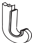
OPTION B Hook Linings a. Bronze/Brass b. Urethane c. Brake Lining (Min. Shaft Dia. = 6")
